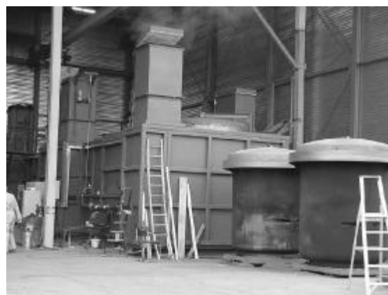
Figure 1 Side view of a Twin-retort carbonisation unit. To the right two carbonisation vessels are shown
